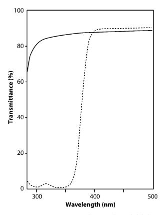
**Fig. 1** Transmittance spectra of near-ambient (solid line, Plexiglass GS 2458) or reduced (dotted line, Plexiglass G 233) ultraviolet screens measured in a spectrophotometer.
